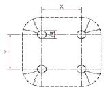
If the centre line spacing, x between two point loads in a row and centre line spacing, y between adjacent point loads in a column are both lesser than 2h (h = thickness of slab), Technical Report TR34 suggests that the quadruple point loads shall be checked for their combined effects.
