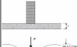
Hetényi's elastic analysis determined that the distribution of bending moment induced by a line load applied to a slab is as shown, with  $M_n=0.21M_p$
